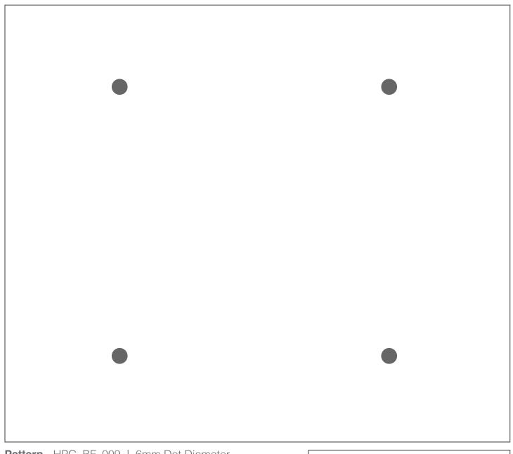
**Pattern** - HPG\_BF\_009 | 6mm Dot Diameter, 101.6mm Gap, Coverage - 0.27%
