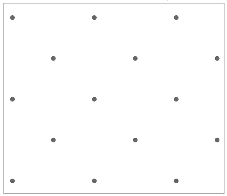
**Pattern** - HPG\_BF\_014 | 4mm Dot Diameter, 70.71mm Gap, S45, Coverage - 0.5%
