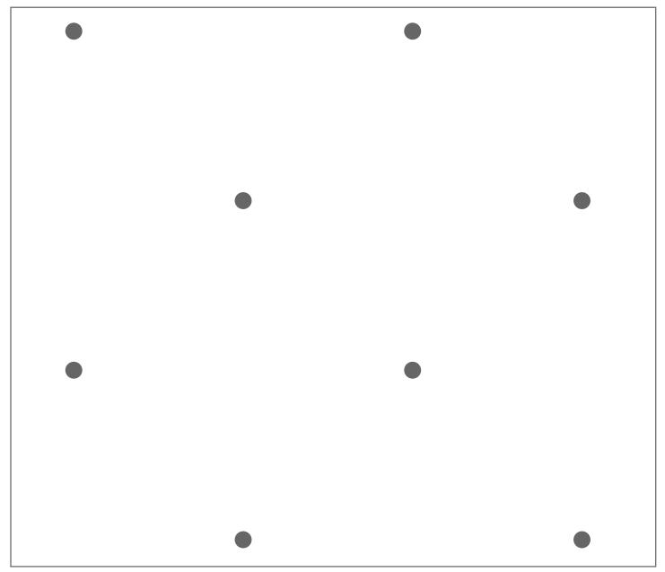
**Pattern** - HPG\_BF\_008 | 5mm Dot Diameter, 100mm Gap, S45, Coverage - 0.39%
