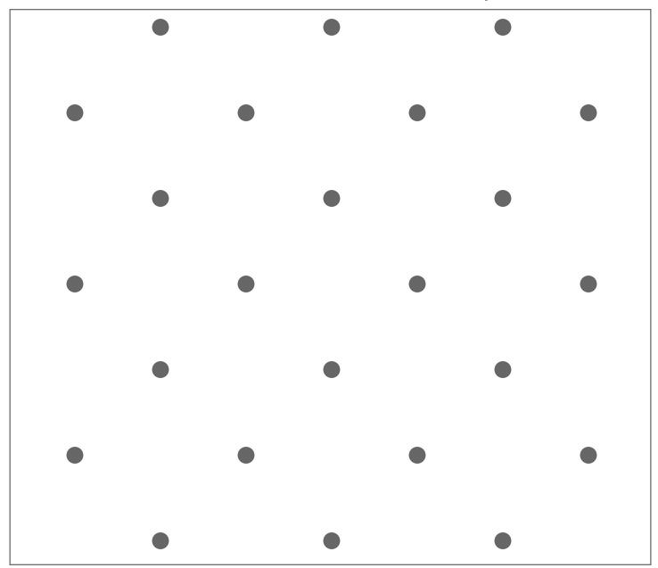
**Pattern** - HPG\_BF\_013 | 5mm Dot Diameter, 2" Gap, S45, Coverage - 1.52%
