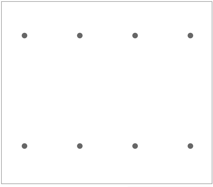
**Pattern** - HPG\_BF\_006 | 5mm Dot diameter, 50mm x 100mm Gap, Coverage - 0.4%
