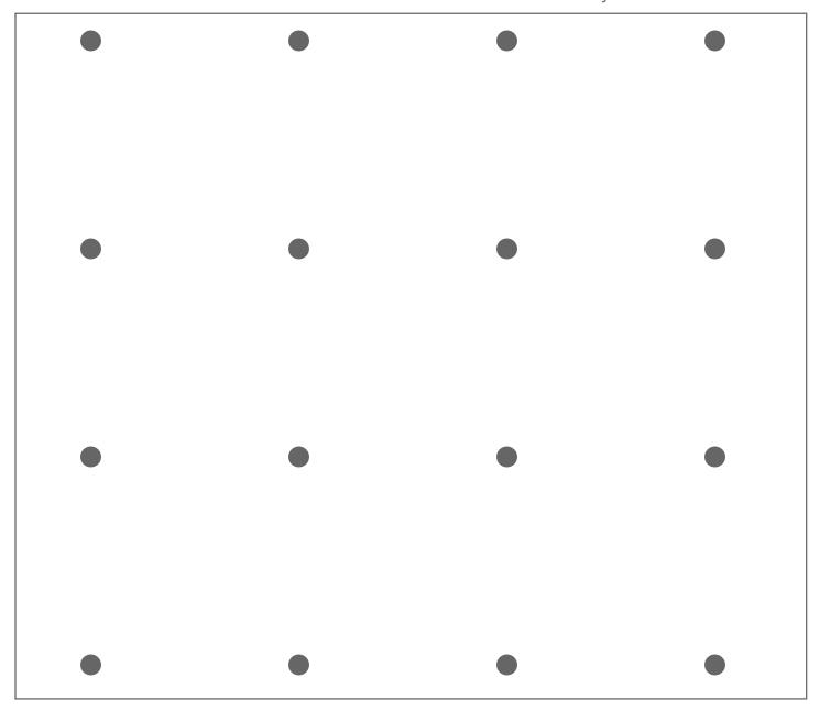
**Pattern** - HPG\_BF\_010 | 5mm Dot Diameter, 50mm Gap, Coverage - 0.79%
