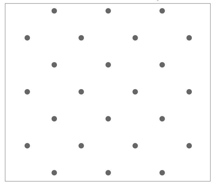
**Pattern** - HPG\_BF\_012 | 5mm Dot Diameter, 50mm Gap, S45, Coverage - 1.57%
